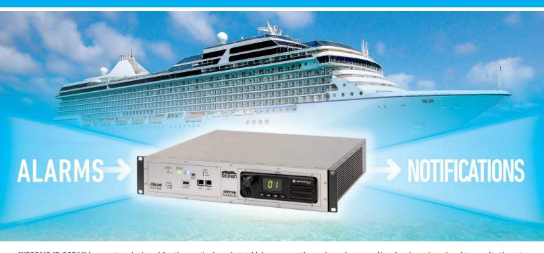
**INFORMO IP OCEAN** is a system designed for the nautical market, which manages the various alarms and/or signals on board and transmits them to staff on the move: for example, on pagers or two-way DMR radios.
